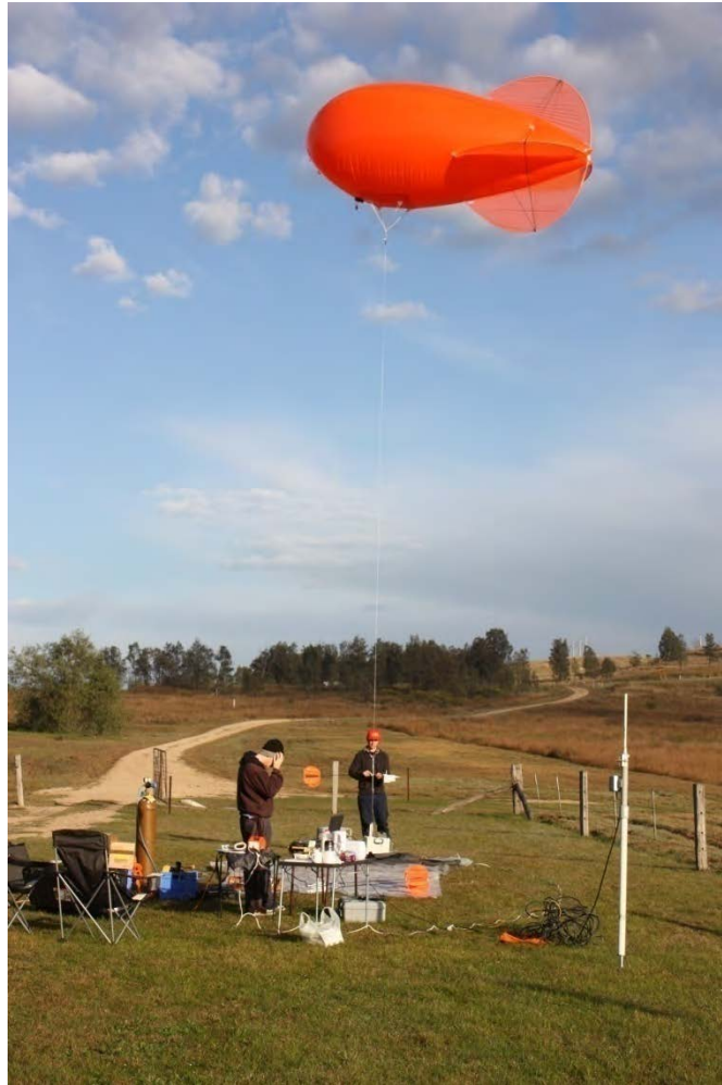
Figure 2. Blimp and tethersonde equipment set-up
