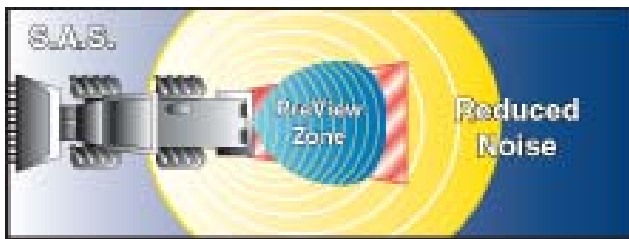
Figure 6.5: Example of the combination of a smart alarm plus proximity sensor [from Preco, 2007].
