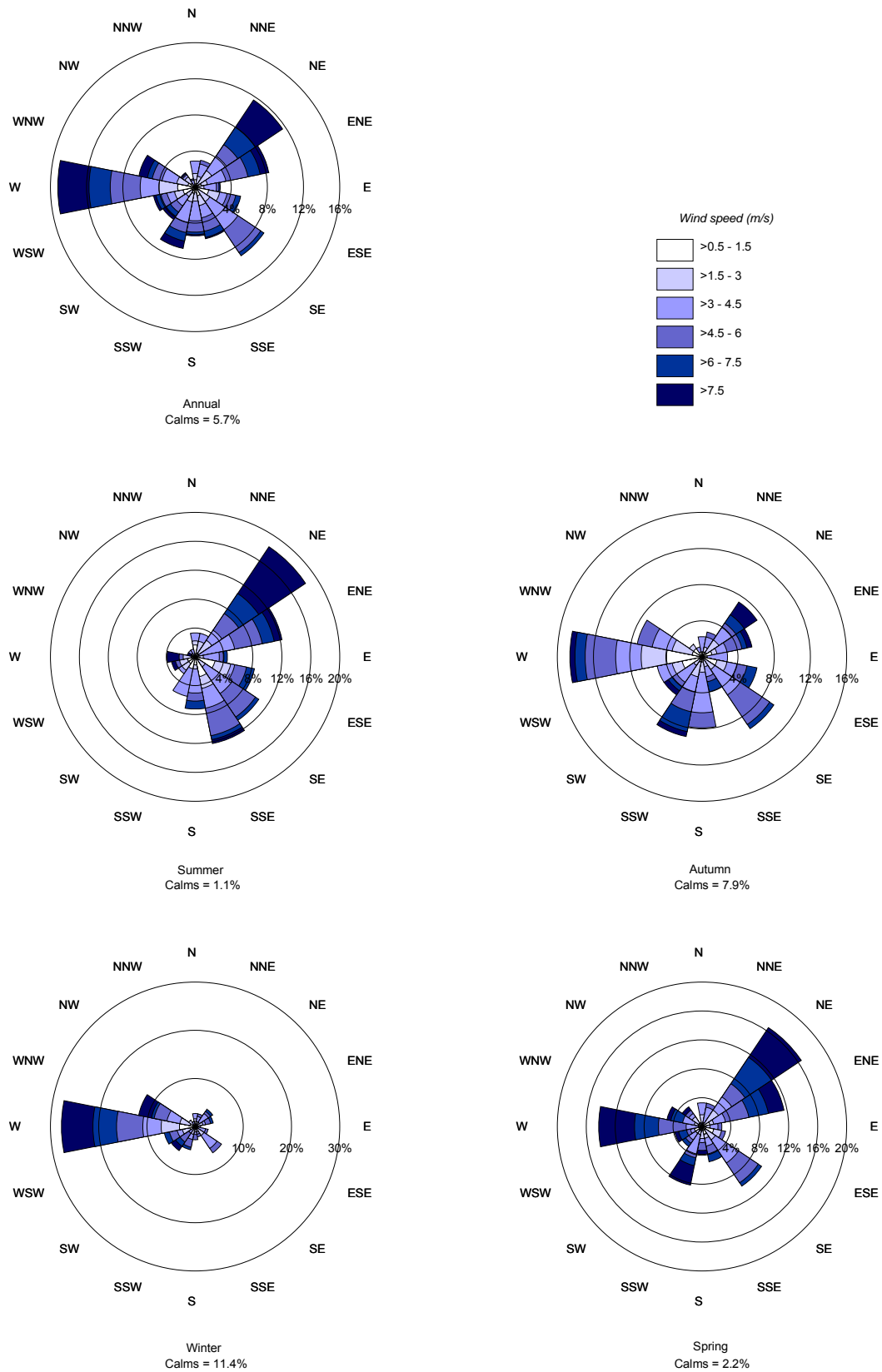
Figure 13: Annual and seasonal wind roses for Kembla Grange (DECCW site) 2001. Day: 9 a.m. and 3 p.m. (Source: Bureau of Meteorology)
