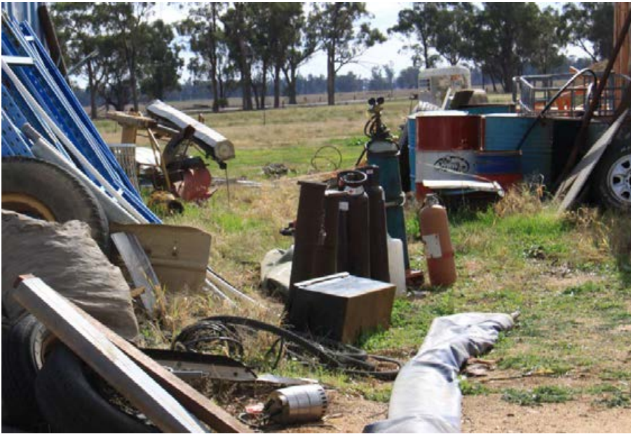
Figure 32 Gas cylinders stored unprotected and near combustible material. Photo: Winston Wickremeratne/EPA
