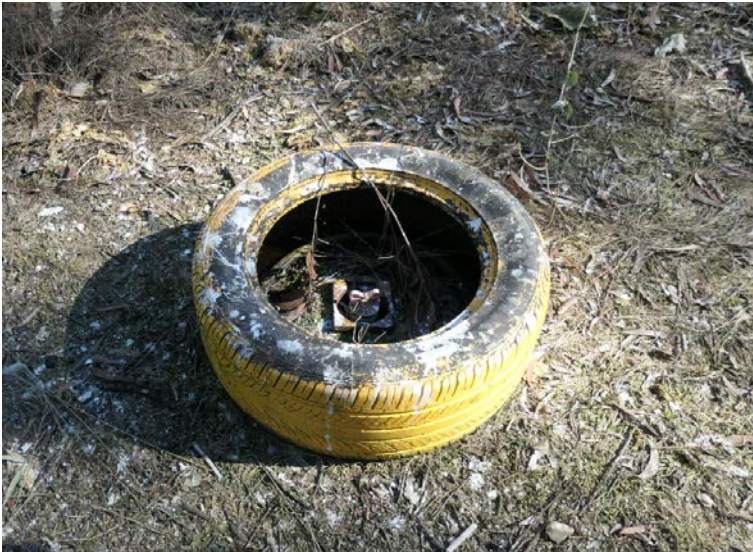
Figure 20 A groundwater monitoring bore with a non-compliant casing. Photo: Karin Schianetz/EPA
