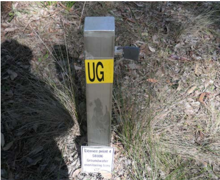
Figure 21 A well-protected, locked and signposted groundwater monitoring bore. Photo: Karin Schianetz/EPA
