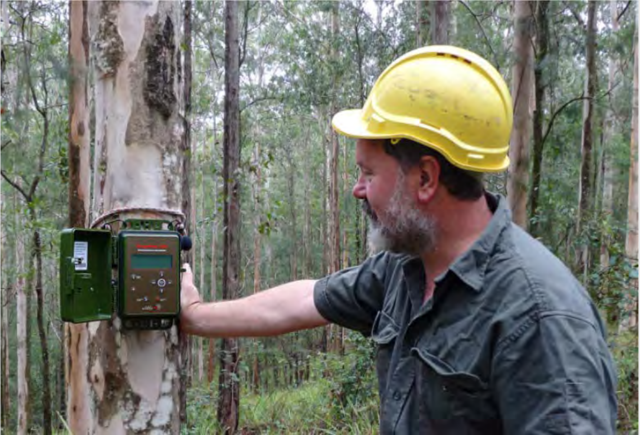
Brad Law from DPI Forestry Science checks a SongMeter used to detect bellows of male koalas. Photo: Forestry Corporation
