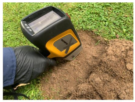
Figure 1 Screening soil with an XRF analyser. Photo: David Langston/EPA
