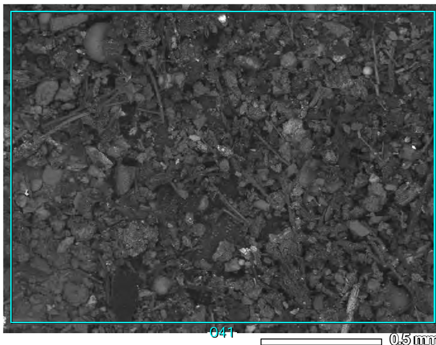
PM16. Stevenson PI Newcastle East Brush (Collected: 09/09/15), UQMP # 13761. An SEM/BSE image of a characteristic overall area selected for SEM/EDS analysis.
