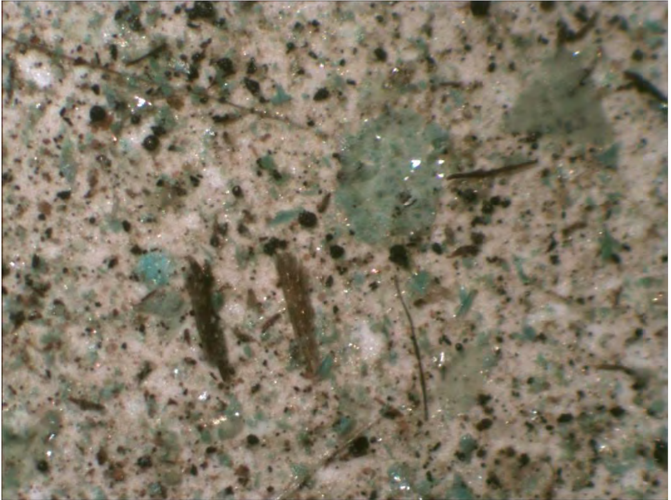
StMPM1. Mayfield East, UQMP # 13173. A stereomicroscopy image of a typical area of the deposit, note that the majority of the particles are encapsulated in polysaccharide slime and copper sludge the green to blue particles.
