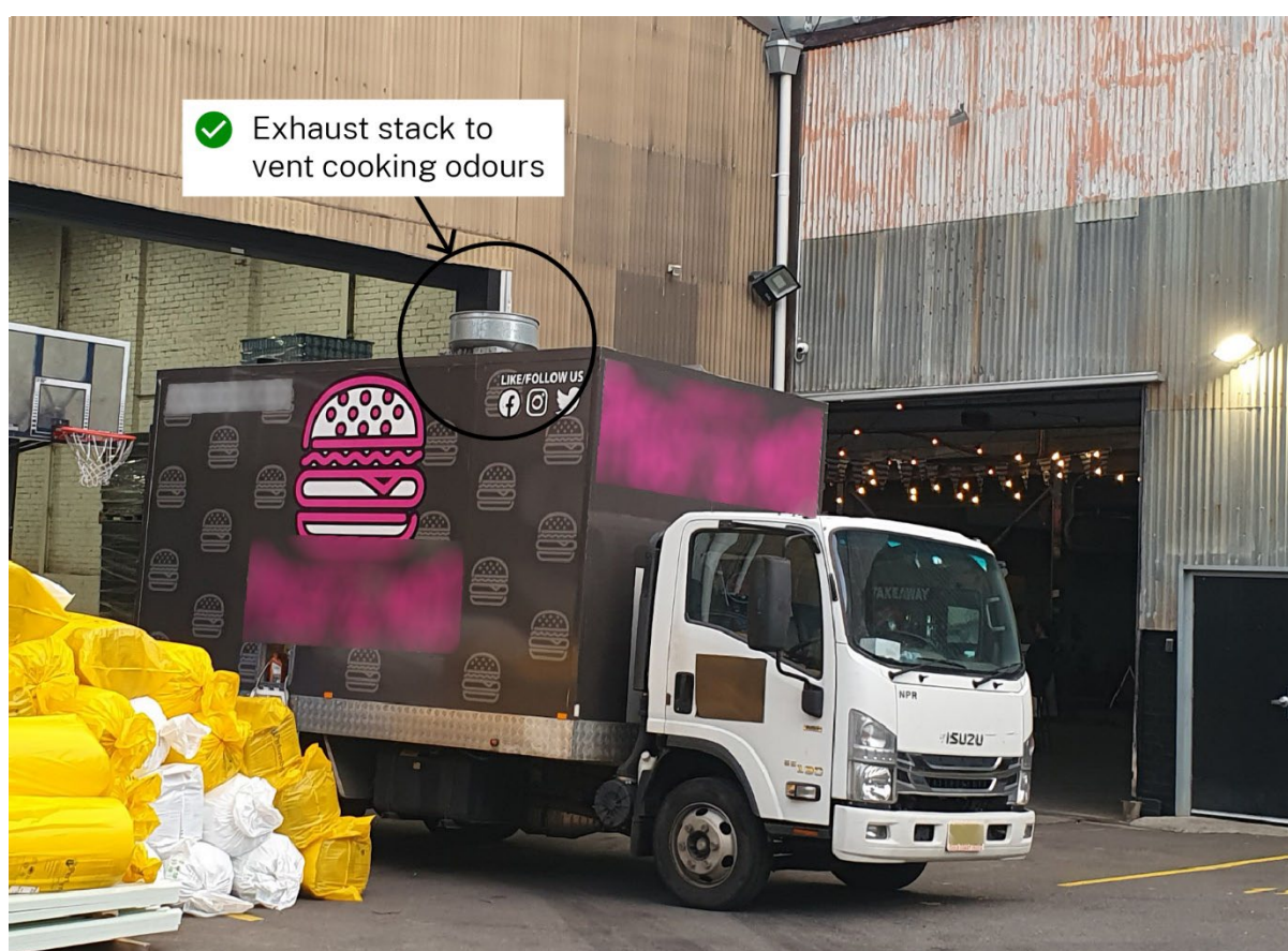
Figure 6 Exhaust stack on a mobile food truck to improve the dispersion of odours Source: Damon Roddis/Zephyr Environmental
