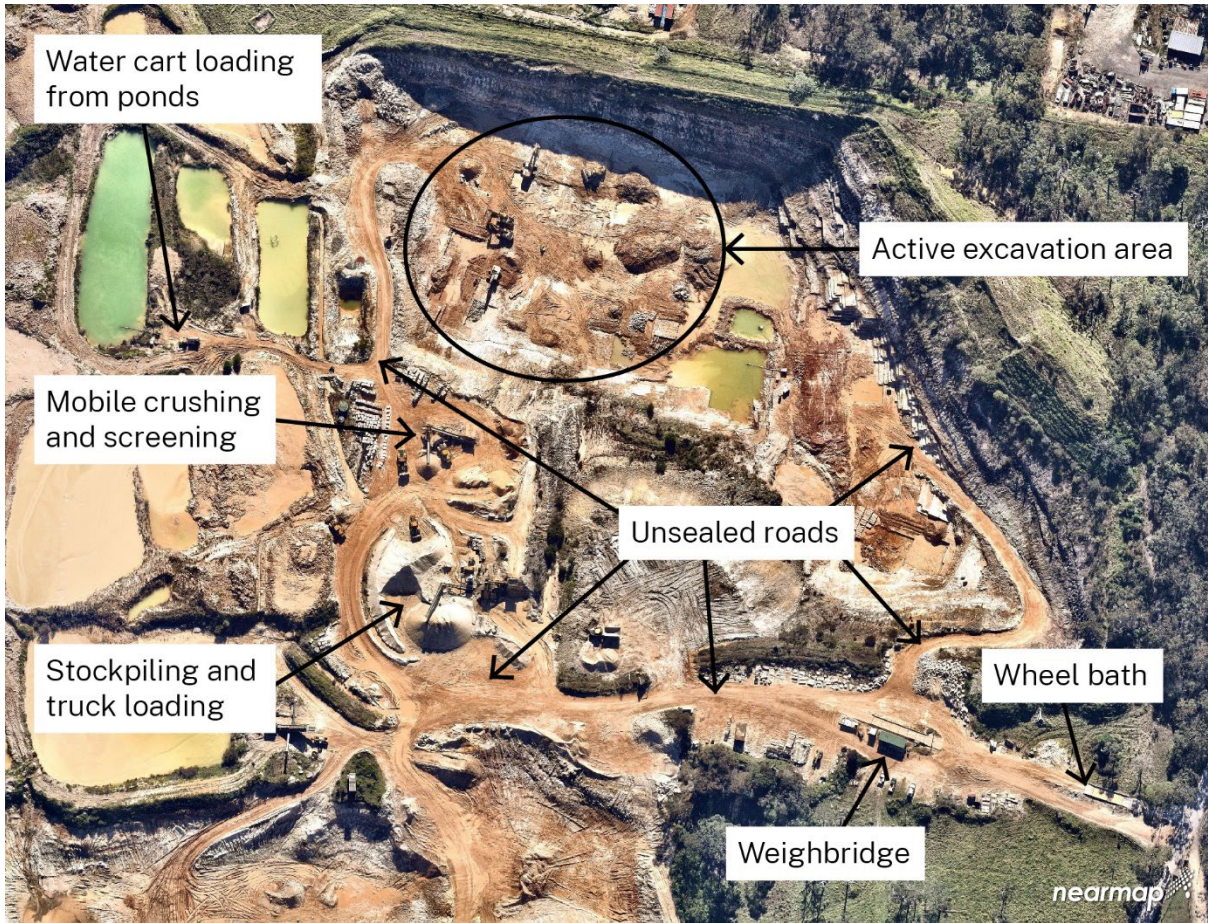
Figure 2 General layout of a quarry site Source: Nearmap aerial image. Overlaid information added by DCCEEW
