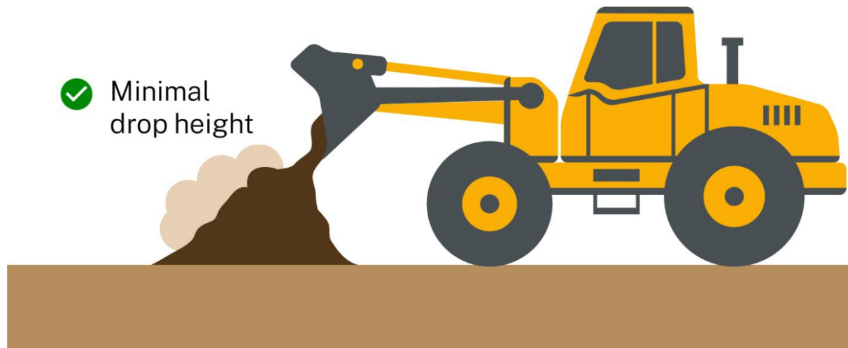
Figure 10 Short drop height from loader to stockpile
