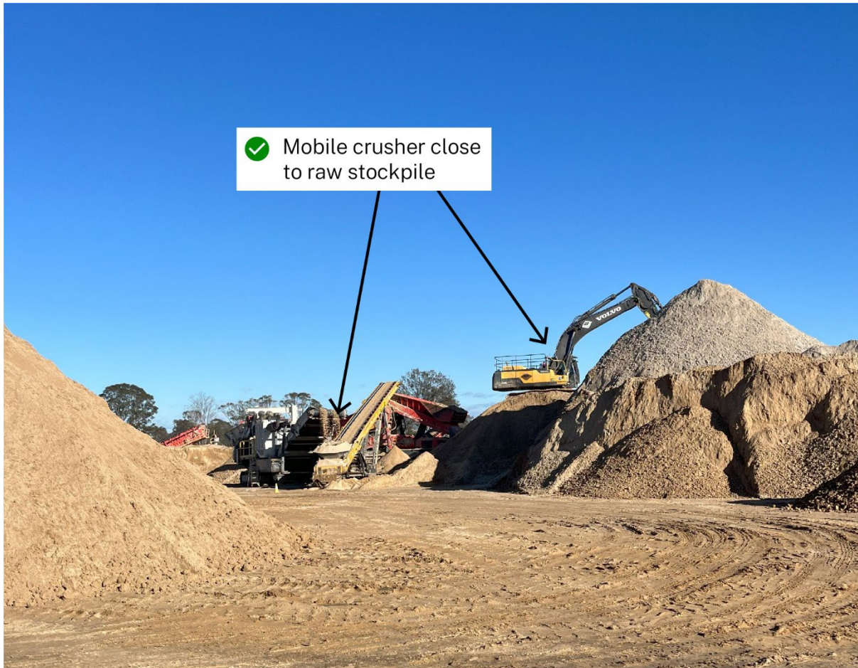
Figure 8 Mobile crusher located close to raw material stockpile Source: Jane Barnett/Zephyr Environmental
