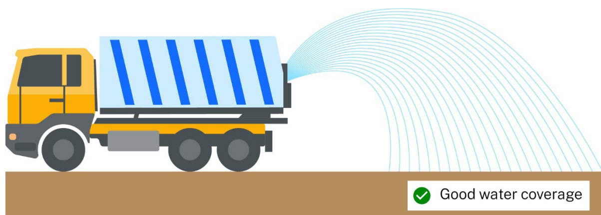
Figure 3 Water cart spraying across the width of the road
