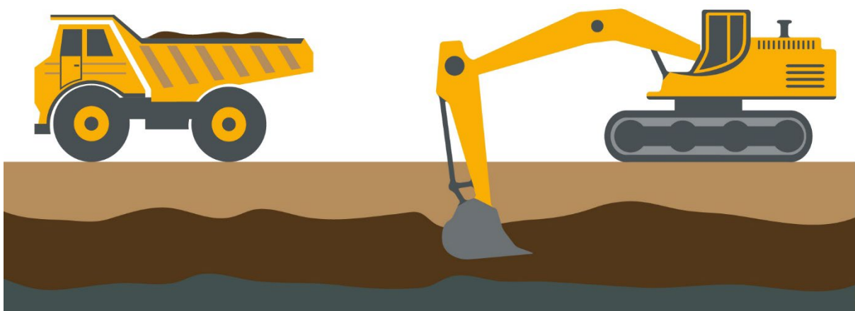
Figure 15 Sludge removal using an excavator
